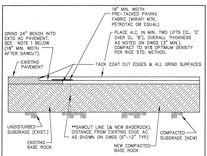
\*\*BENCH GRIND REQUIREMENT SHOWN DOES NOT REPLACE ANY REQUIREMENT NOTED ON DRAWINGS FOR SAWCUT BACK FROM EDGE OF EXISTING AC & INSTALLATION OF NEW BASEROCK. BENCH GRIND REQUIREMENT APPLIES AFTER ALL EXCAVATION & BASEROCK PLACEMENT (PRIOR TO PAVING), TO AVOID FULL DEPTH AC JOINTS.
